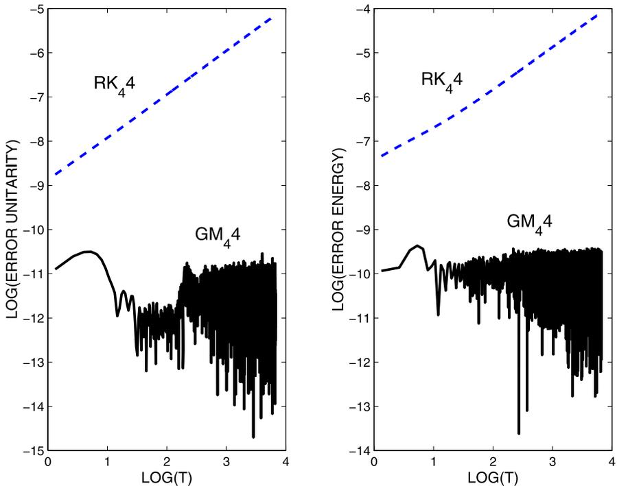
**Fig. 3** Error in the preservation of unitarity and energy as a function of time in double logarithmic scale for the nonsymplectic RK<sub>44</sub> and symplectic splitting GM<sub>44</sub> methods applied to the Schrödinger equation. Both 4-stage explicit fourth-order methods are used with the same time step
